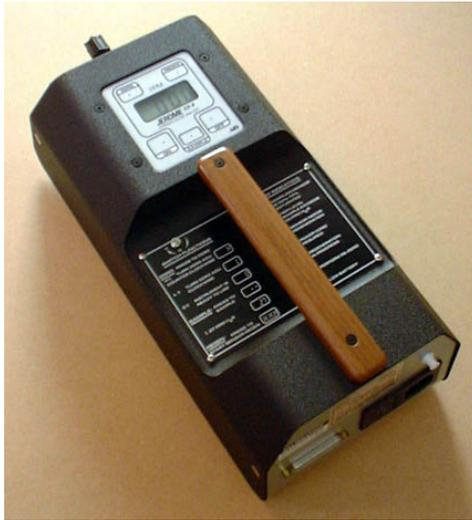
Figure 4-7. Hydrogen Sulfide Monitor (Jerome 631-x) (Courtesy of Arizona Instruments)
