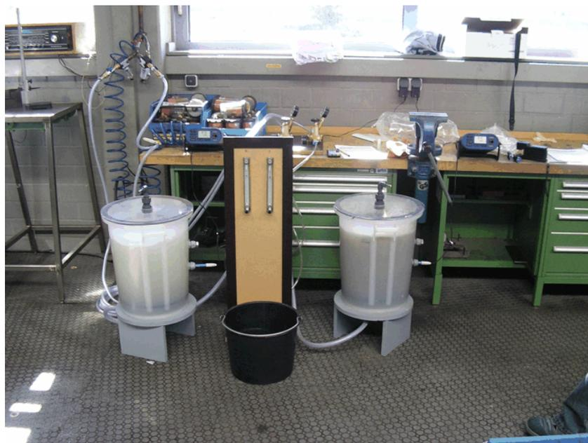
Figure 4-6. Odor Emission Capacity Test Reactors
