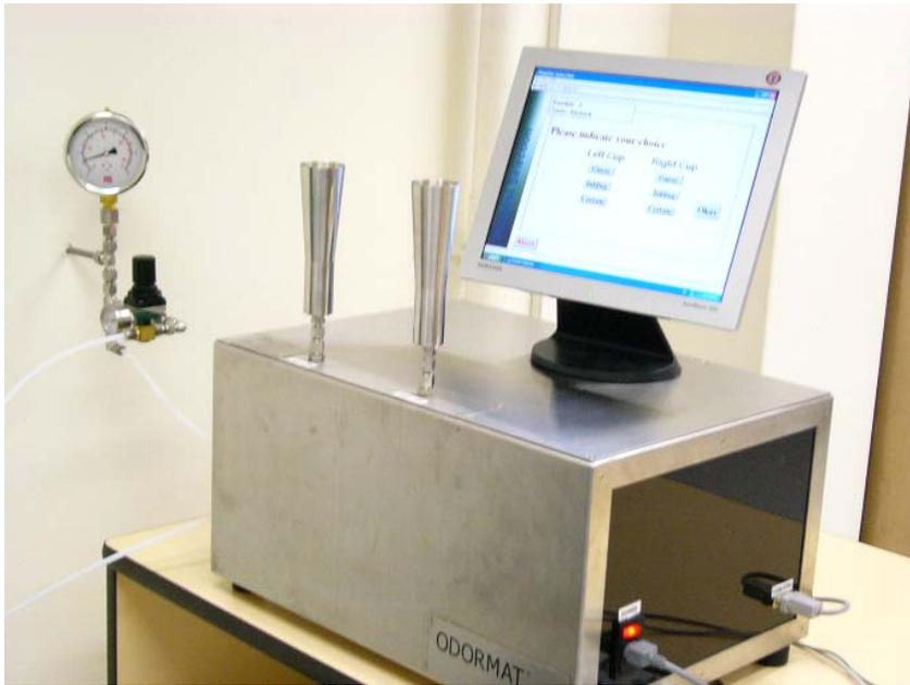
Figure 4-4. Example of Olfactometer with Two Sniffing Ports (Courtesy of Aromatrix, Singapore)
