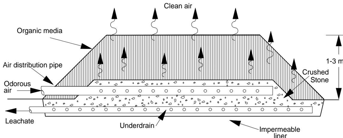
Figure 8-5. In-Ground Organic-Media Biofilter
