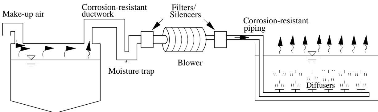
Figure 8-8. Activated-Sludge Scrubbing System
