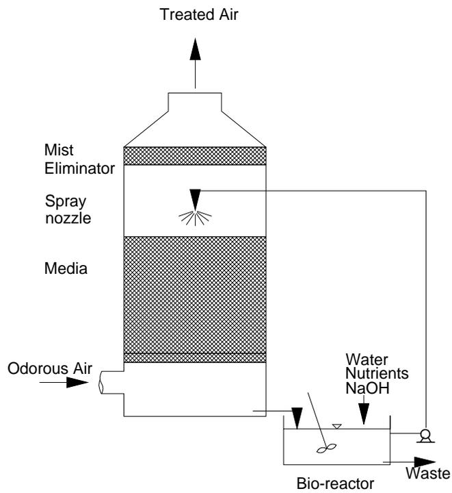
Figure 8-6. Biological Scrubber Systems: Biotrickling Filter (top) and Bioscrubber
