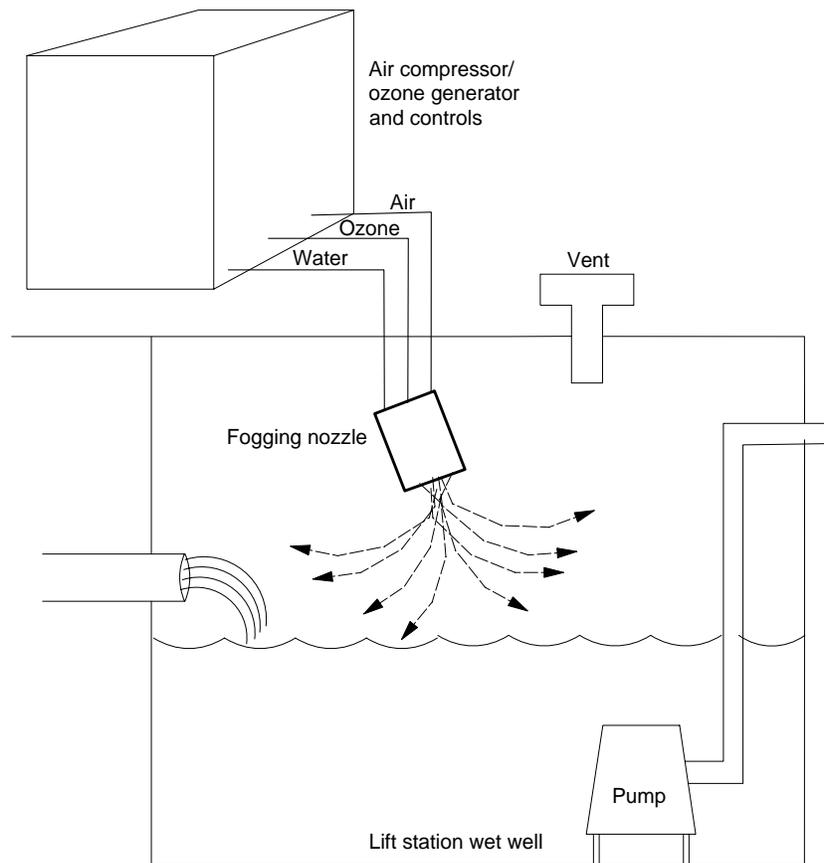
Figure 8-10. Hydroxyl Ion Fog Process
