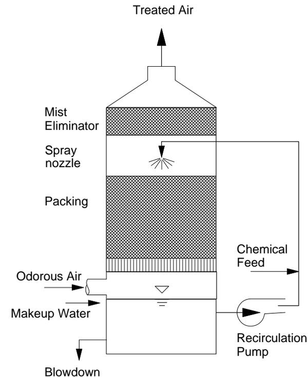
Figure 8-3. Packed Tower Chemical Scrubber
