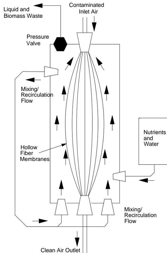
Figure 8-9. Schematic of Hollow Fiber Membrane Reactor
