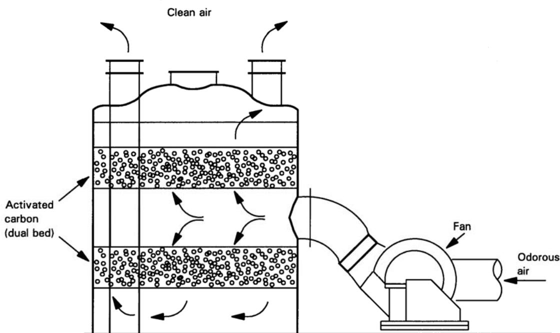
Figure 8-4. Dual-Bed Activated-Carbon Adsorber
