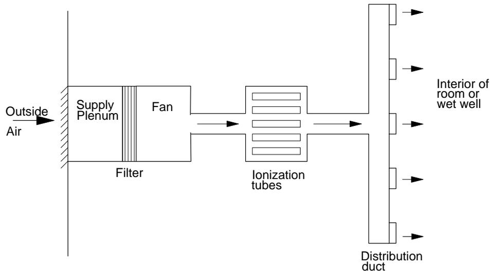
Figure 8-7. Air-Ionization Process
