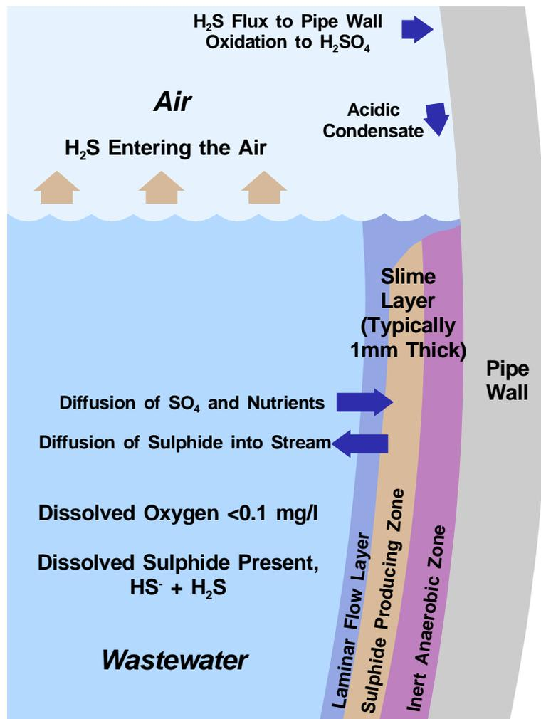
Figure 9-2. Overall Corrosion Mechanism in Wastewater Pipelines (from ASCE, 1989)
