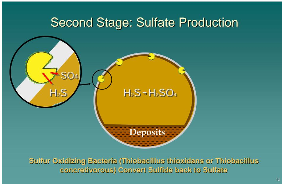
Figure 9-3. Second Phase of Corrosion: Sulfate Production
